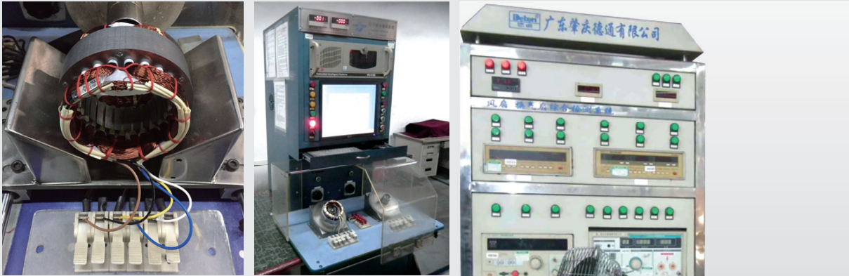
Coil inspection one by one
